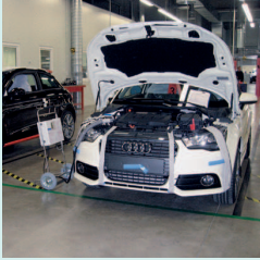
Aushärtebereich Teileverklebung Hardening area for cars that have had new items glued on
